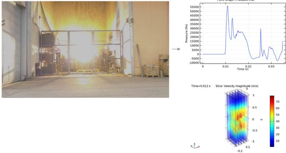
Figure 2 - Short circuit tests and pressure measurements and simulation performed at AIT Austrian Institute of Technology GmbH
