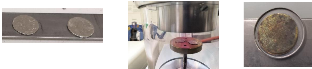
Figure 18: Sputtering Au onto Li foil for passivation (left: 2x pristine Li chips; central: in sputtering; right: passivated Li foil)
